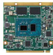
Portwell's PQ7-M109 is designed with latest Intel Atom®/Celeron®/Pentium® processor (codenamed Elkhart Lake), featuring 2x graphic performance and 1.5x overall CPU performance improvement than previous generation platform.
