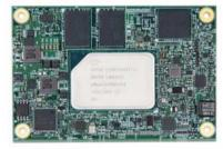
PCOM-BA02GL, a Type 10 Mini COM Express® (84 x 55mm) module is based on Intel Atom® x6000E and Pentium® N and J Series Processors, featuring LPDDR4-3200 MT/s on board memory, dual 4K display.
