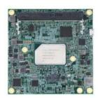
Type 6 compact COM Express® (95 x 95 mm) module which based on Intel Atom® x6000E and Pentium® N and J Series Processors
