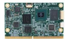
The PSMC-M840 SMARC 2.1 module is designed with NXP i.MX 8M Plus family processor, featuring high graphic performance and great memory bandwidth.
