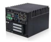
Intel® desktop W480E chipset and 10th Generation Intel® Core™ i3/i5/i7/i9 processors technologies that can support dual DDR4 memory, three Gigabit Ethernet ports, one M.2 E Key socket, one Mini-PCle socket and 3x PCle Expansion Slot option.
