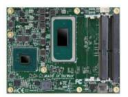
COM Express® Type VI Basic Module with 11th Gen Intel® CoreTM Processors (Tiger Lake-H) DDR4, PCIe Gen 4, USB 3.2 Gen 2, 2.5 Gigabit TSN Ethernet, SATA III, TPM 2.0, DDI, eDP/LVDS and VGA
